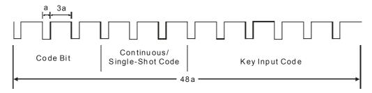
The diagram above shows the basic transmitting waveform. A basic transmitting waveform consists of 12-bits serial data.
